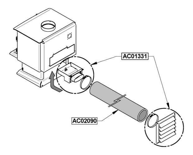
If you wish to draw combustion air through the floor, fix the angled plate with the oval outlet such that the outlet faces the floor.
