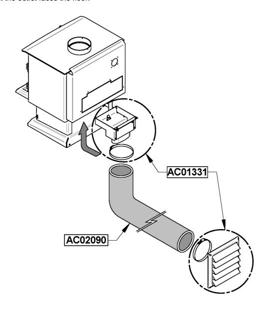
Position the adapter underneath the stove. Align the two fixation holes on the adapter with those located on the stove's rear heat shield. Fix the adapter into place with the two supplied screws.
