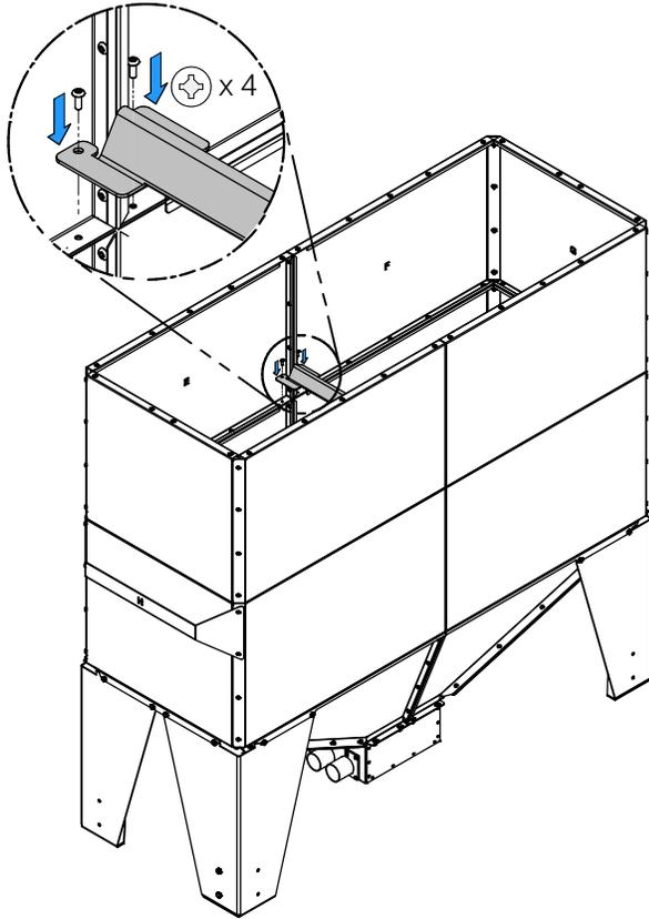
8. Reinstall the upper section, the stiffener with the screws.
