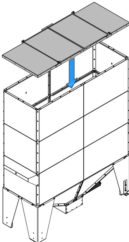
10. Secure the tank top panels with the screws removed previously.
