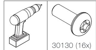
6. Screw the four corners together. Seal corners with silicone.
