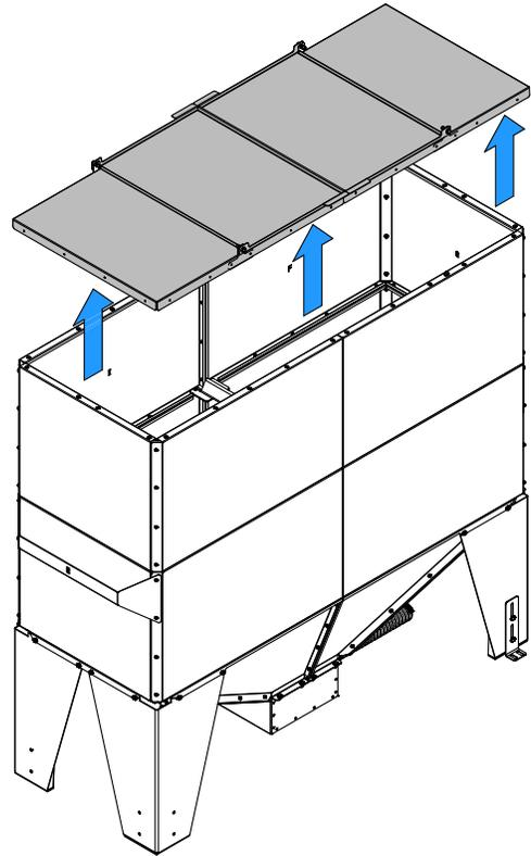
2. Remove the upper section, the stiffener and the screws from the base.
