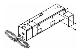
2. Use the four screws provided to attach the other end of the brackets to the rear heat shield of the stove. The louvers should be at the bottom of the fan housing.
