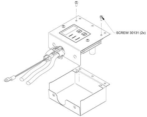
Secure the PC board assembly to the PC board bracket (see Figure 6).
