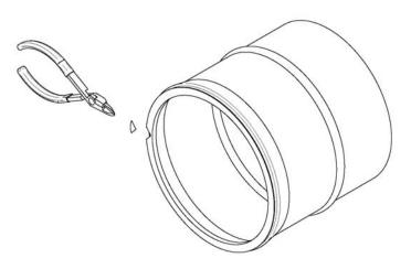
Align the adapter notch with the fireplace warm air outlet notch and turn until the flange is fully inserted. The adapter is well in place when its flange is completely inserted and the adapter can rotate freely.
