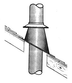
flashing to the roof using roofing nails. Place the storm collar over the chimney and the flashing. Tighten it with the bolt supplied making sure that the joint is properly caulked.
