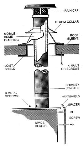
(h) Fit the roundtop raincap with the spark screen to the top of the chimney.
