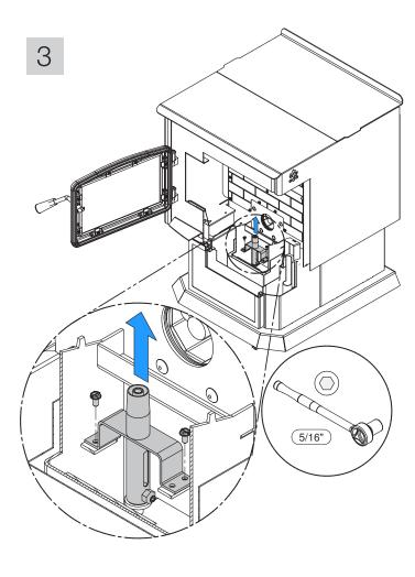
Pull the igniter upwards to gain access to the connector
