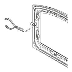
Figure 11: Removing the split pin
