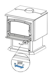
On the other hand, too much air can make the fire uncontrollable, creating very high temperatures in the unit as well as in the chimney and seriously damaging them. A reddish glow on the unit and on the chimney components indicates overheating. Excessive temperatures can cause a chimney fire.
