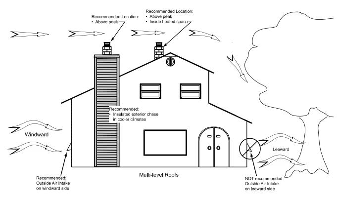
Figure 19: Air supply in conventional houses
