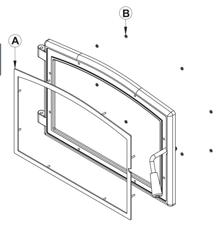
Note: It is not necessary to remove the glass to install the overlay.
