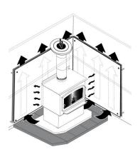
It is often desired to use as little space as possible when installing a wood stove. To do this, it is possible to reduce the clearances safely and install the stove closer to the walls by permanently installing a heat shield between the stove and the flammable material.
