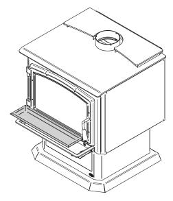
Figure 7: Installing the ash lip pan
