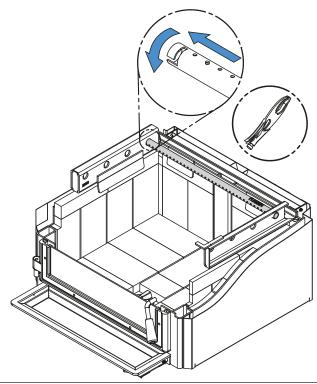
Note that secondary air tubes **(B)** can be replaced without removing the baffle board **(A)** and that all tubes are identical.
