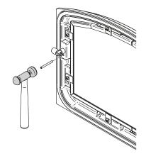
Figure 12: Installing the split pin
