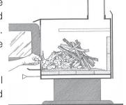
Once the fire has ignited, the door can be closed with the air control still fully open. When the kindling is almost completely burned, standard firewood pieces can be added.
