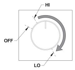
Figure 21: Variable speed control
