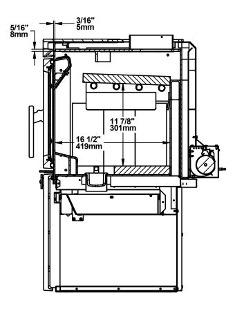
Figure 6: Side view - Combustion chamber
