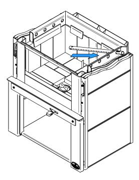
1. Starting with the rear tube, lean and stove the right end of the secondary air tube into the rear right channel hole. Then lift and stove the left end of the tube into the rear left channel.
