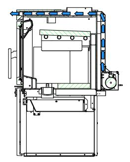
A blower is already installed on this stove The blower is installed on the back of the stove to increase the airflow through the heat exchanger and improve hot air circulation in the room. When used regularly, the blower can provide a small increase in efficiency, up to 2%. However, the use of a blower should not be used as a way to gain more output from a stove that is undersized for the space it is intended to heat..
