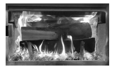
Close the primary air control by small increments (ex: 1/16 of an inch), from  $\frac{1}{2}$ " to fully closed, between 4 and 15 minutes after the loading period. Before closing further, make sure the flame intensity is increasing or stable. Close the air control completely. Turn ON the blower at maximum speed.
