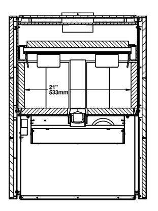
Figure 5: Front view - Combustion chamber
