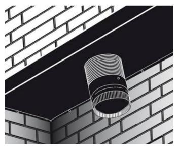
Figure 28: Block-off Plate
