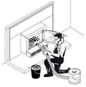
The chimney should be checked regularly for creosote build-up. Inspection and cleaning of the chimney can be facilitated by removing the baffle. See <u>«Appendix 4. Air Tubes and Baffle Installation»</u> for more details.
