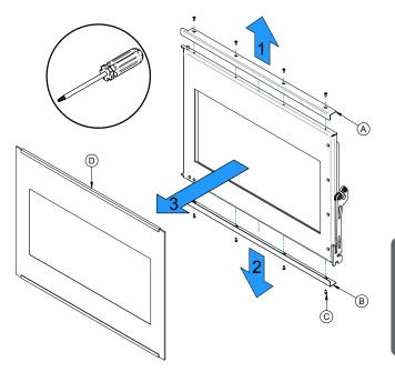
Figure 22: Replacing the glass
