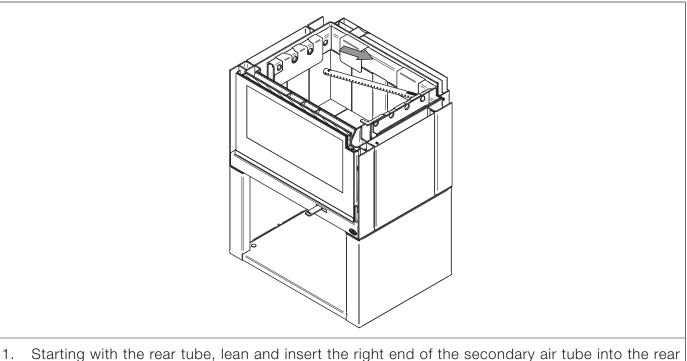
right channel hole. Then lift and insert the left end of the tube into the rear left channel.
