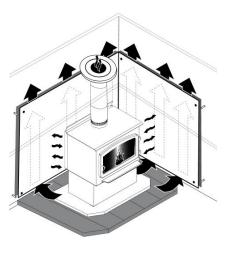
Figure 35: Heat shield
