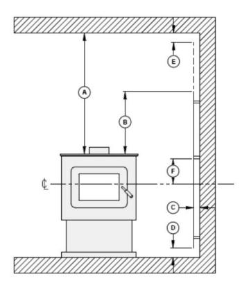
Figure 36: Heat shield clearances
