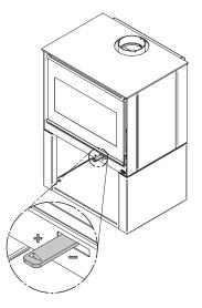
Figure 21: Air Intake Control
