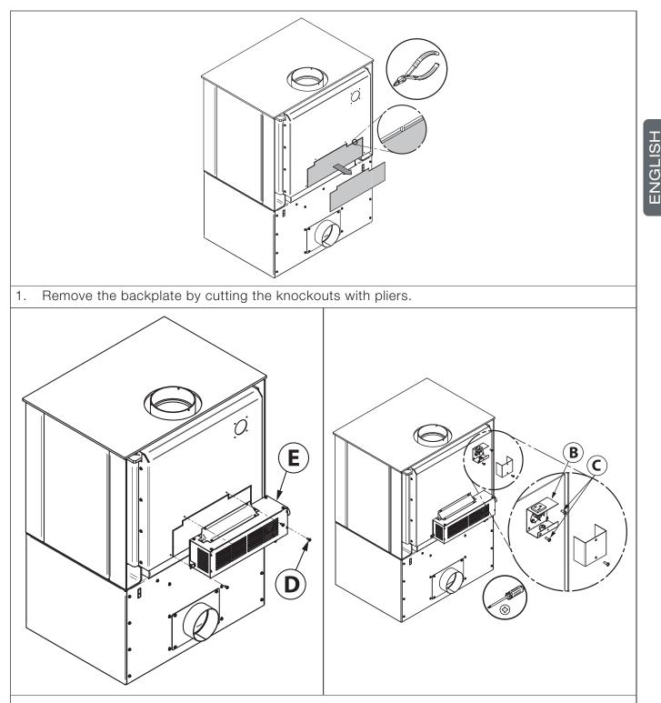
2. Screw the blower **(E)** in place using the screws **(D)** included in the installation manual. Screw the thermodisc **(B)** with the screws **(C)** supplied with the thermodisc on the back of the stove.
