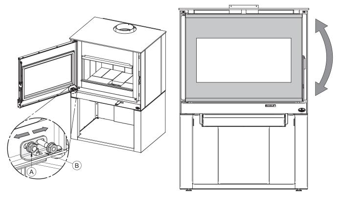
Figure 28: Door angle adjustment
