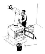
The chimney should be checked regularly for creosote build-up. Inspection and cleaning of the chimney can be facilitated by removing the baffle. See <u>«Appendix 7. Air Tubes and Baffle</u> <u>Installation»</u> for more details.
