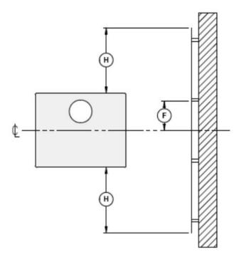
Figure 37: Heat shield clearances
