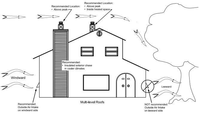
Figure 41: Air supply in conventional houses
