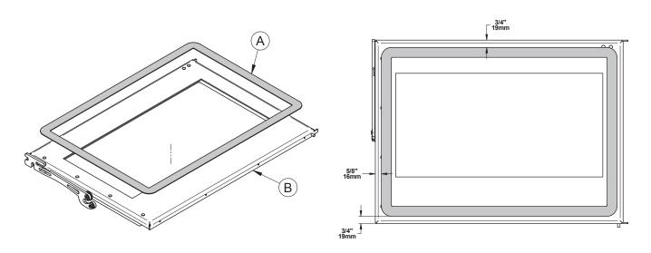
Figure 24: Replacing the glass gasket
