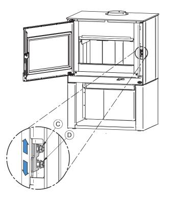
Unscrew the nuts (D) and lift the door latch mechanism (E) to increase the pressure on the door. Lower the mechanism (E) to release pressure.
