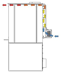
Figure 18: Air flow with a blower
