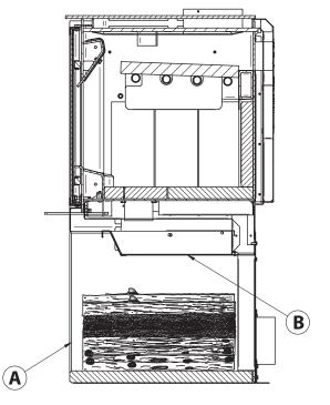
Figure 20: Wood storage underneath the stove
