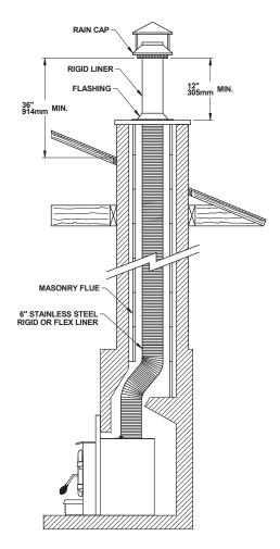
Figure 23: Liner Installation
