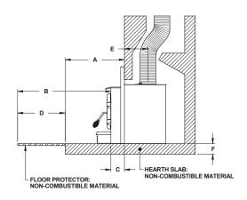
Figure 18: 5" or less raised base installation
