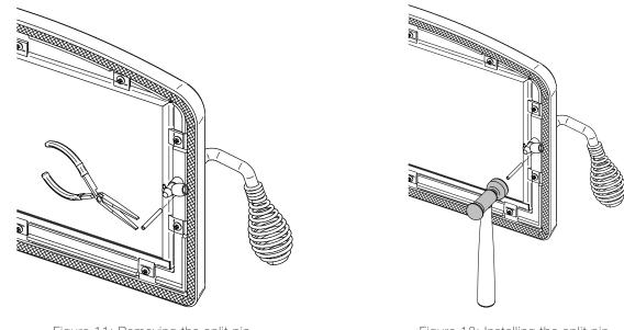
Figure 11: Removing the split pin
