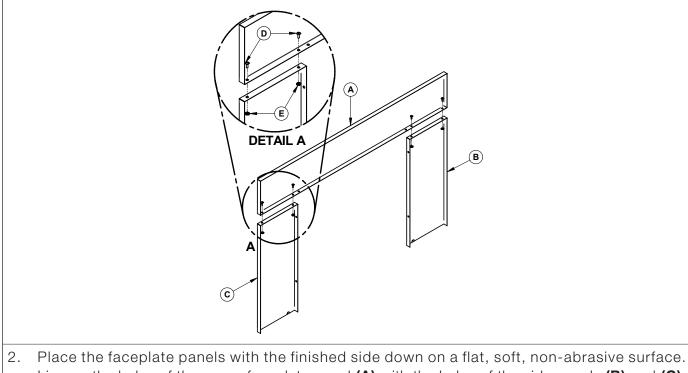
Place the taceplate panels with the finished side down on a flat, soft, non-abrasive surface. Line up the holes of the upper faceplate panel (A) with the holes of the side panels (B) and (C). Secure them together using four bolts (D) and nuts (E) provided.
