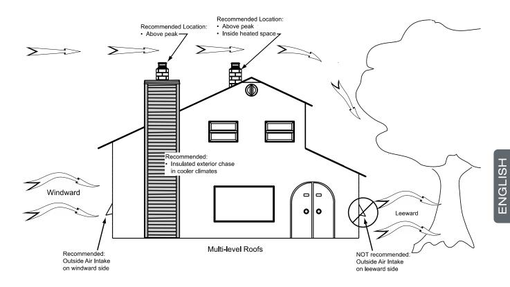
Figure 30: Air supply in conventional houses
