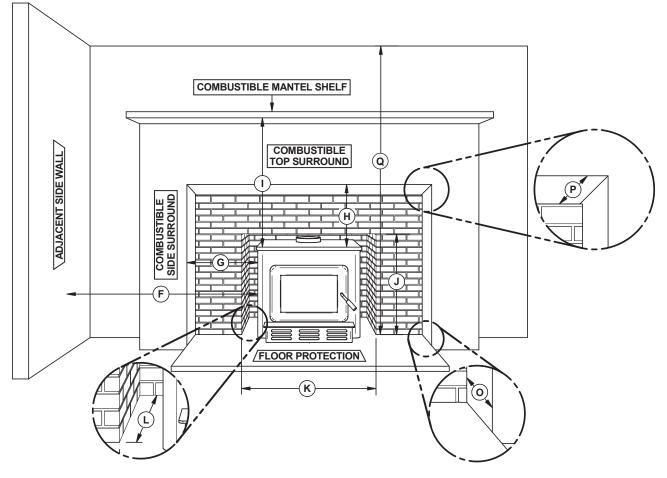
Figure 20: Masonry Opening and Clearances
