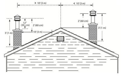
Figure 28: Minimum Chimney Height
