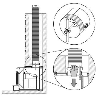
Figure 25: Liner fastening system
