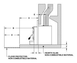
Figure 19: More than 5" raised base installation
