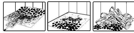
Remove ash first, and then rake charcoal towards the front of the firebox before loading so that it will ignite the new load.
