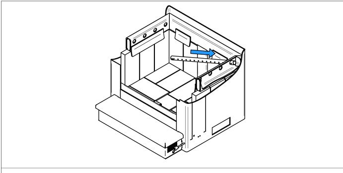
1. Starting with the rear tube, lean and insert the right end of the secondary air tube into the rear right channel hole. Then lift and insert the left end of the tube into the rear left channel.
