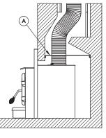
Figure 21: Block-off Plate
