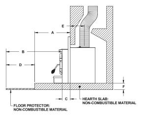
Figure 17: Additional Floor Protection
