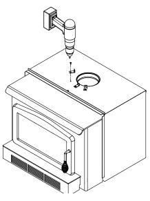
Figure 26: Securing the brackets
