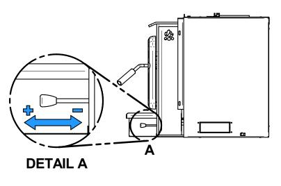
Figure 10: Air Supply Control
