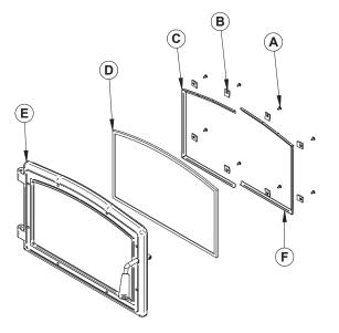
Figure 13: Replacing the glass
