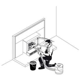
Before installing the firebrick, check to ensure that none are broken or damaged in any way, and replace the damaged ones. Check the firebrick for damage at least annually and replace any broken or damaged ones with new ones. Inspection and cleaning of the chimney is facilitated by the removable baffle.
