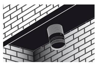
Figure 22: Block-off Plate
