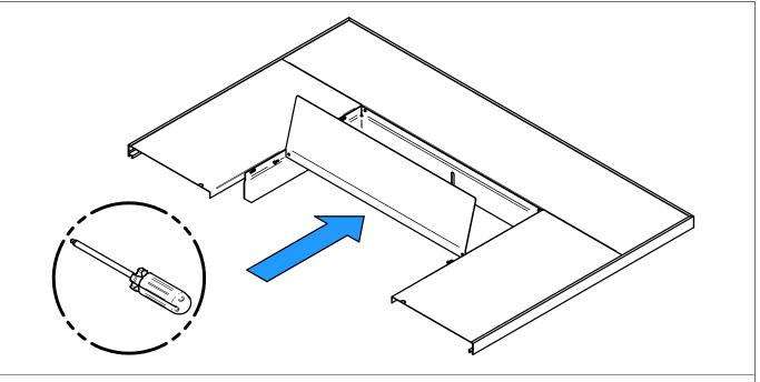
1. Install the heat shield on the faceplate (assembled with the faceplate extension) using 3 selfdrilling screws included in the kit. The heat shield should be pointing upwards.
