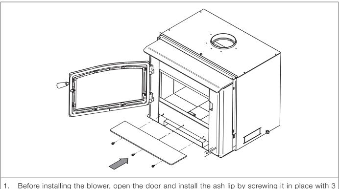
1. Before installing the blower, open the door and install the ash lip by screwing it in place with 3 screws, located in the user manual kit.
