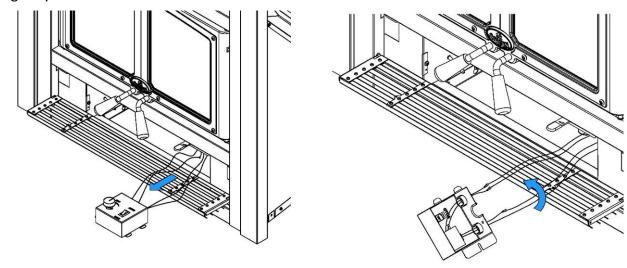
Unplug the wires. Also unplug the wire located on the terminal by removing the screw holding it in place.
