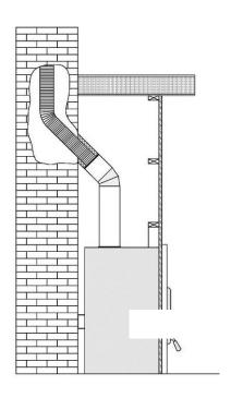
Connection to a masonry chimney
