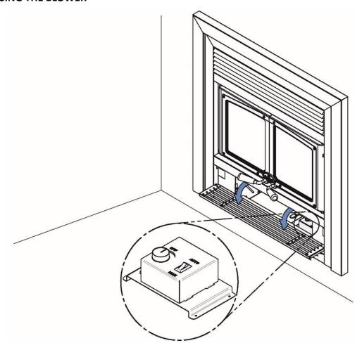
The EVEREST fireplace is equipped with a blower and a control box, accessible by pulling down the lower louvre of the faceplate.
