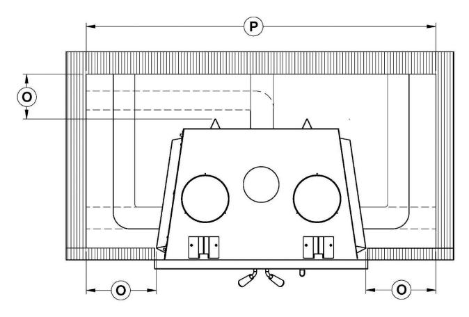
The framing dimensions are for reference only. These are recommended measurements to avoid duct to be within the standoff and have too sharp pipe angles. Smaller dimensions may be obtained depending on pipe size, type or run configuration.
