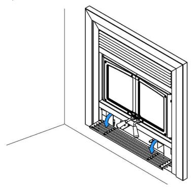
Remove the screw securing the blower control box to the fireplace.
