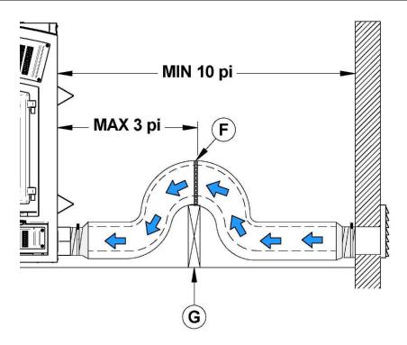
To complete the installation, make a hole of 1/4" to 1/2" (6 mm à 13 mm) bigger than the insulate pipe diameter in the outside wall of the house at the chosen location. From outside, place the outside wall termination (E) in the hole (open side down) and fasten the register to the wall, with screws.
