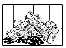
Remove ash first, and then rake charcoal towards the front of the firebox before loading so that it will ignite the new load.
