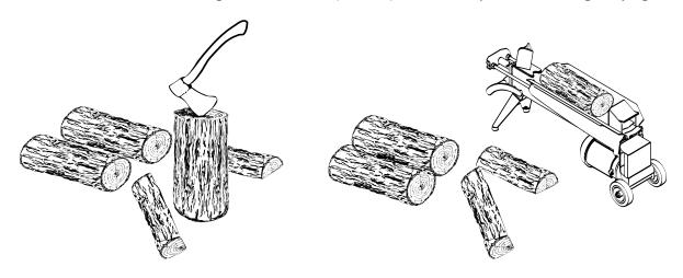
Wood should be split to a range of sizes, from about 3" to 6" (75 mm to 150 mm) in cross section. Having a range of sizes makes starting and rekindling fires much easier. Often, the firewood purchased from commercial suppliers is not split finely enough for convenient stoking. It is sometimes advisable to resplit the wood before stacking to dry.
