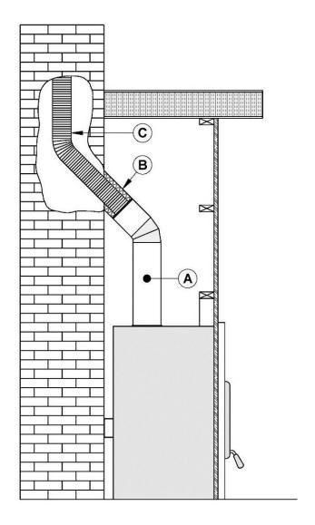
Note: Make sure the liner exceeds at least 12" (30 cm) the top of the masonry chimney.
