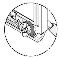
3. Reinstall the split pin (A) with a small hammer.
