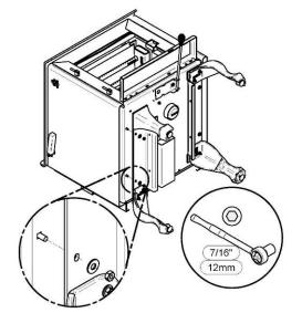
5- Secure both leg support assembly to the underside of the firebox using the bolts, washers and nuts removed in **step 3**. Supports can be installed on either side.
