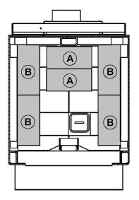
For transportation purpose, the top bricks have been laid on the bottom of the firebox. It is mandatory to install them on the brick supports before you operate the stove. Failure to install the bricks as describe bellow may result in stove damage and will void warrantee.
