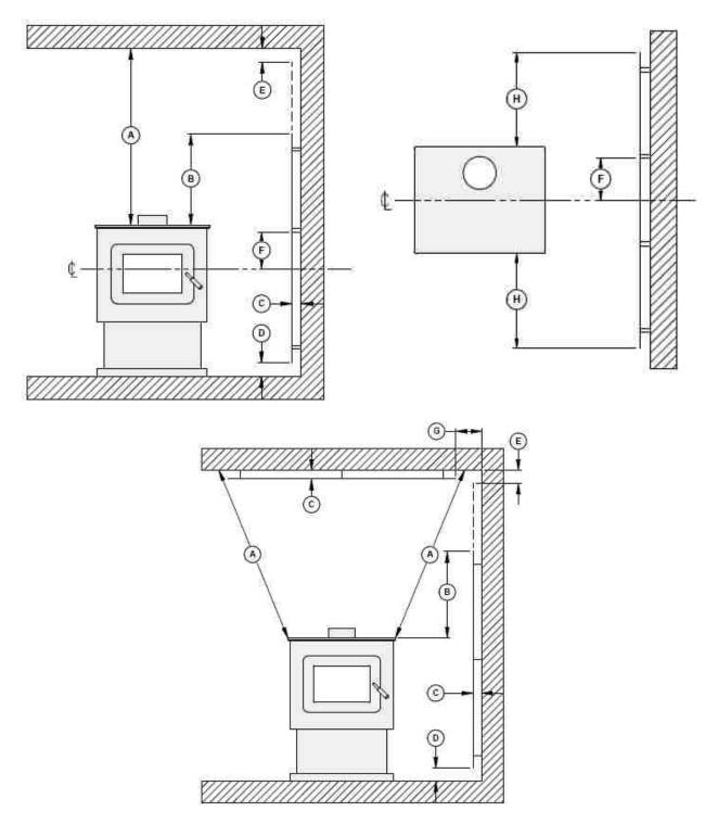
**Clearances for shield construction**
