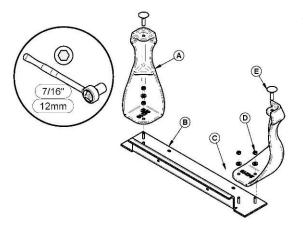
4- Secure each leg (A) on support (B) using (2) washers (C) and (2) nuts (D) supplied in the kit. Repeat the same mounting procedure for the second support.
