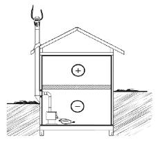
**Good System Design** Inside chimneys are preferred because even when no fire is burning, there is normally upward flow in the system.
