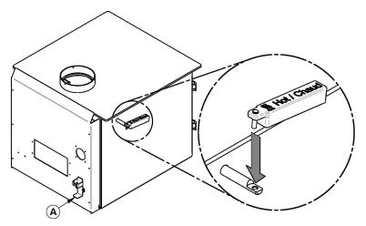
CAUTION: THE HANDLE CAN BECOME VERY HOT. GLOVES ARE REQUIRED TO HANDLE THE BYPASS DAMPER.
