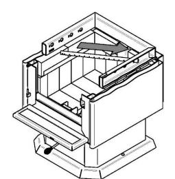
1- Starting with the rear tube, lean and insert the right end of the secondary air tube into the rear right channel hole. Then lift and insert the left end of the tube into the rear left channel.
