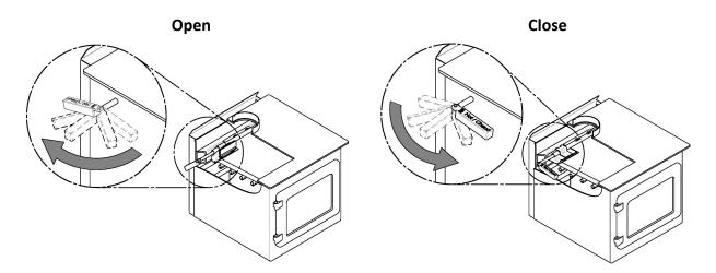
CAUTION: NEVER LEAVE THE REMOVABLE HANDLE INTO THE SMALL ROD EXTENSION UNLESS YOU ARE BUILDING A FIRE OR RELOADING THE UNIT. THE HANDLE SHOULD BE REMOVED FROM THE STOVE AT ALL OTHER TIMES AND PLACED ON ITS HANDLE SUPPORT (A).
