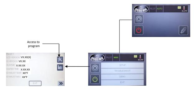
Page 1 provides information on the software version of the stove's two electronic cards. In addition, you have the total number of hours your stove has been in operation, the temperature of the exhaust gases and the maximum temperature that your stove has reached.
