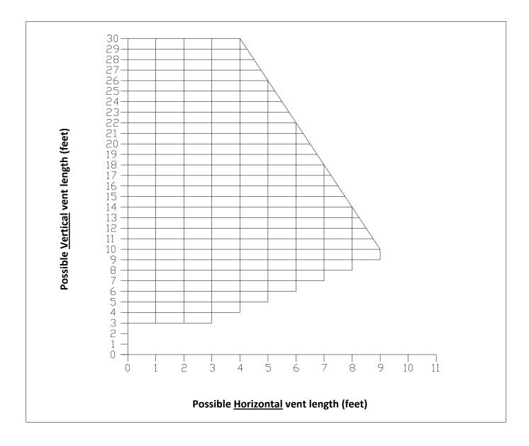
For example, let's imagine an installation consisting of a horizontal vent coming out at the back of the stove on a total distance of 8 feet. This horizontal run is followed by a tee and a 6-foot vertical rise. This type of installation is not acceptable. As you can see, the vent termination is clearly outside the allowed configuration zone on the chart because the venting system proposed <u>does not have at least one</u> foot of vertical rise for each foot of horizontal run.
