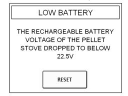
If you use a 24V auxiliary battery system, the pellet stove will stop when the tension of the batteries goes below 22.5V. This is made to increase battery life.
