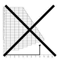
Instead, if the installation consisted of a horizontal vent coming out at the back of the stove on a total distance of 4 feet, followed by a tee and a 6-foot vertical rise, it would be acceptable. The termination is within the allowable configuration zone on the chart since it would have at least one foot of vertical rise for each foot of horizontal run. Furthermore, the total vertical rise is at least 3-feet high.
