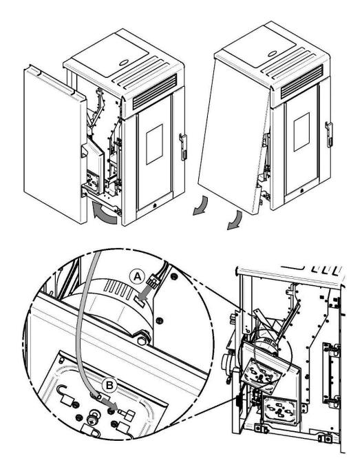
Unplug the blower connections **(A)** and the silicone tube **(B)**. Unplug the temperature sensor **(C).**
