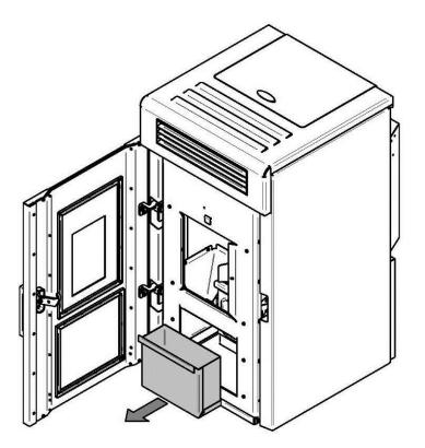
2. Empty the ash drawer and vacuum around the drawer and also at the bottom of the combustion chamber.
