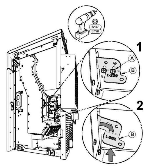
Remove the faulty thermal switch. Replace new thermal switch (D) underneath the bracket (B) by means of 2 screws (C).
