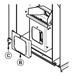
5. Verify that the clean out trap gasket is still in good condition; replace it if needed (3/16" black round gasket (AC06815)).
