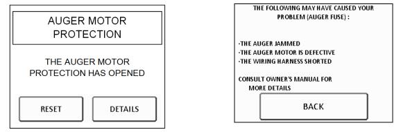
The auger is jammed or auger motor failed. Go to the troubleshooting page (see Section 9.2: Testing components) on the LCD touch screen and test auger motors. If one of the motors is not running check if motor is defective or jammed.
