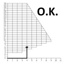
Instead, if the installation consisted of a horizontal vent coming out at the back of the stove on a total distance of 4 feet, followed by a tee and a 6-foot vertical rise, it would be acceptable. The installation end should be within the allowable configuration zone on the chart since it would have at least one foot of vertical rise for each foot of horizontal run. Furthermore, the total vertical rise would be at least 3-foot high.
