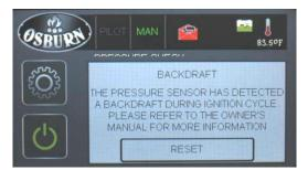
Your stove is equipped with a digital pressure sensor that measures your chimney draft. At startup, if the pressure is negative and less than -0.1 inches water column (eg. -0.15), this informative message will appear. When the exhaust blower starts, if the pressure becomes positive, the stove will start normally. Negative pressure can be cause by kitchen or bathroom hood.
