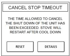
This error is also called the double-click error. If you press on the stove's stop button inadvertently, you have 15 seconds to press on the start up button for the stove to continue to work normally. If you wait more than 15 seconds, this message will appear and the stove will stop. It will ignite again automatically after its cool temperature is reached.
