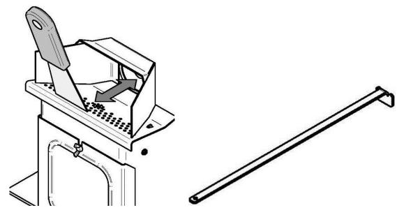
2. The burn pot (A) simply sits onto the air intake channel. You must lift to remove it from the stove. Two small pins guide the burn pot in place. Make sure that the burn pot is well in place before turning on the stove (as shown in the diagram).
