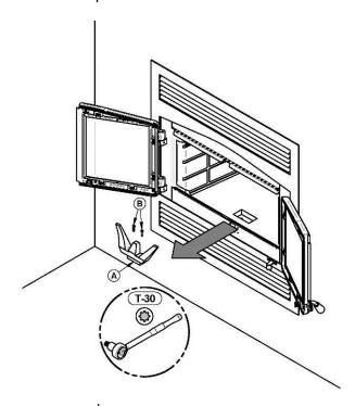
2- Remove the floor refractory slab (C).
