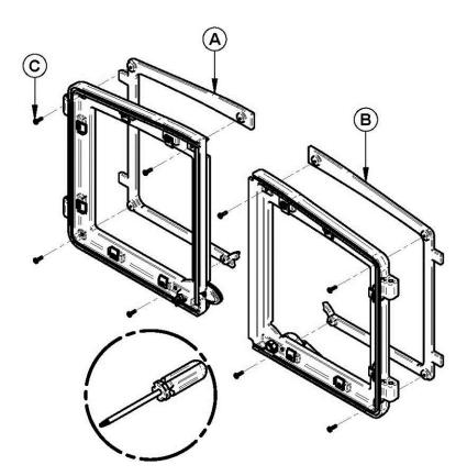
Position the overlays (A) and (B) on the door frames and secure them from the inside of the doors using the 8 included screws (C).
