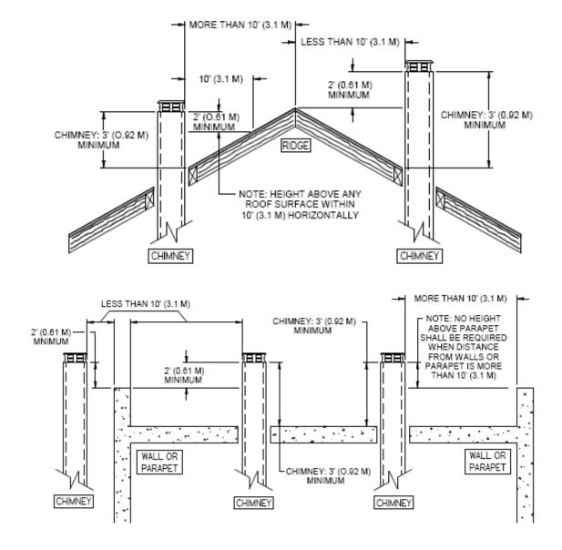
12. For installations where more than one chimney is located in the same non-chase or within the same area, we suggest that their terminations be separated by at least 16" (410 mm) horizontally, and 18" (460 mm) vertically. This separation is to prevent smoke migrating from one chimney to another.
