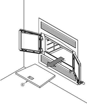
2. Remove the floor refractory slab (C).
