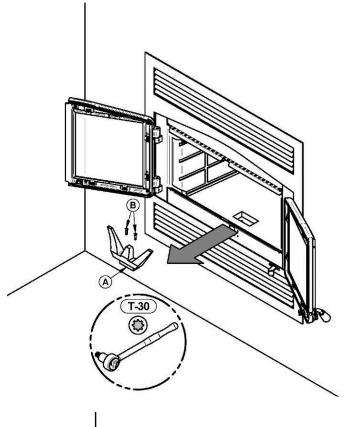
1. Using a ratchet key and a Torx (T-30), unscrew the two Torx screws (B) holding up the andiron (A).
