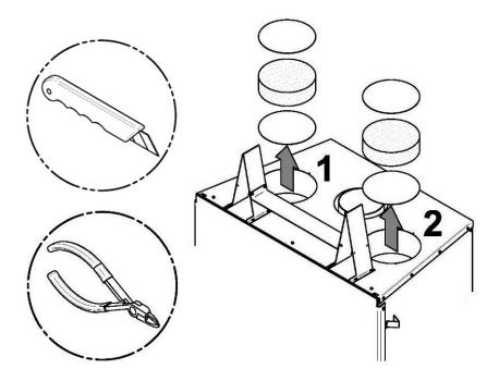
2. Secure the 6 steel brackets (B) with 6 screws provided (C) on top of the fireplace (3 for each ducting). Insert the ducting (A) (not provided) into each opening and secure it in place using the steel brackets (B) installed previously with 6 other self-tapping screws provided (C).
