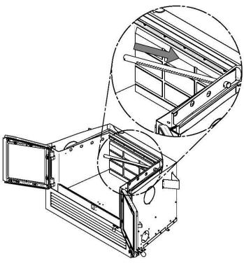
4. Starting with the rear tube, lean and insert the right end of the secondary air tube into the rear right channel hole. Then, lift and push the tube towards the right inside the hole in the right channel.
