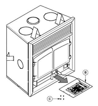
3. Remove and keep the heat shield (B) and the 4 screws (C).
