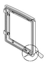
Turn the handle counter clock wise one turn to increase pressure. To reduce the pressure, when installing a new gasket for example, turn clock wise.
