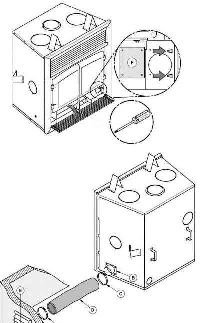
Flip the fireplace's lower decorative louver. Install the blocking plate (F) included in the kit, on the front opening of the air control housing. Using a screwdriver, secure with two screws.
