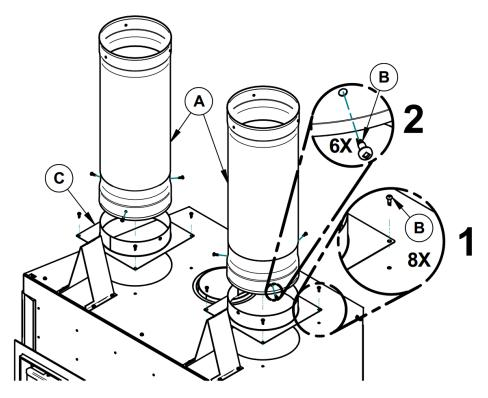
Secure the telescoping sections (A) to the heat distribution box (C) with self-tapping screws (B) (3 per telescoping section). Determine the needed height and secure the two parts of the telescoping sections together with 3 self-tapping screws provided. Insert the adjustable frame (D) in the heat distribution box (C), press it against the non-combustible finishing material and secure with 4 screws into the heat distribution box. Set the decorative plate (E) to the adjustable frame (D).
