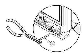
3. Re-install the split pin with a small hammer.
