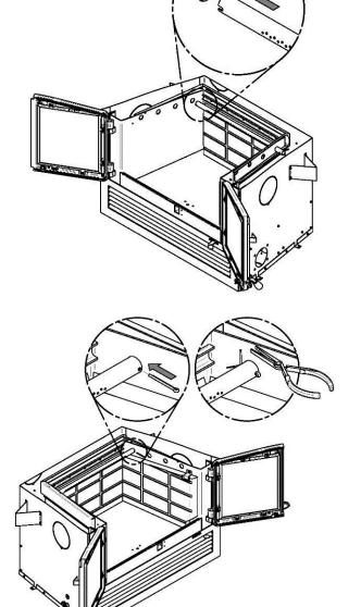
5. Align the notch in the left end of the tube with the tab of the left air channel hole.
