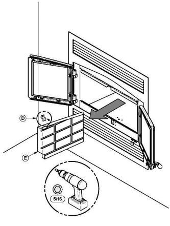
3. Using a power screwdriver and hex tip 5/16", remove the slab holder (D) and the left refractory slab (E).
