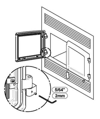
Using a flat screwdriver, turn the adjustable hinge rods in the direction shown to adjust the doors. Tighten all door hinge pressure screws when they are at the desired positions.
