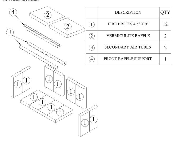
Figure 4.2 – Firebrick layout for Osburn 1100 Insert model
