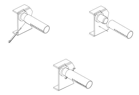
Figure 4.3 – Secondary Air Tube replacement
