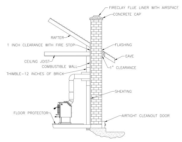
Figure 1.7 Connection to a Masonry Chimney (Exterior Shown)
