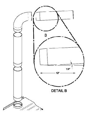
FIGURE 2.3 (B) Minimum Slope
