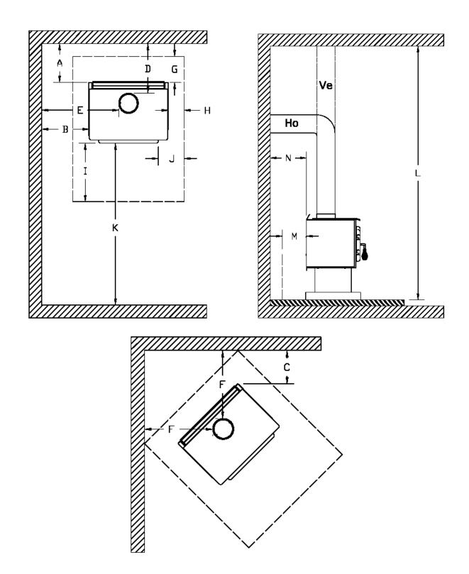
FIGURE 1.3 Clearances to combustible materials and floor protection
