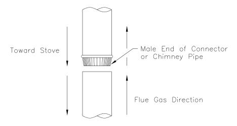
FIGURE 2.3 (A) Connecting Sections
