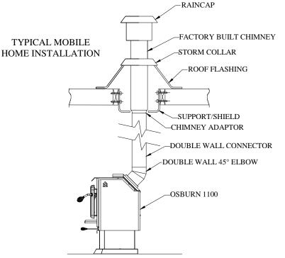
Figure 1.1 Necessary installation components.
