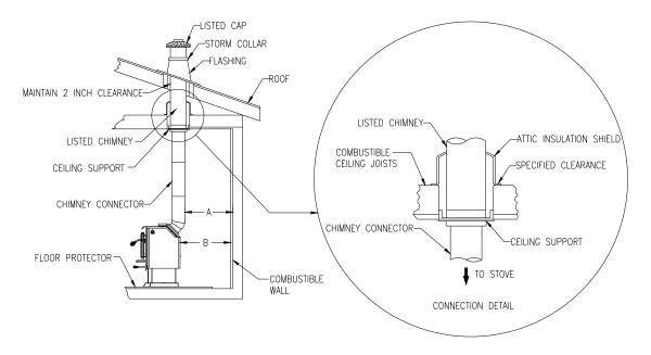
Figure 1.8 Connections to a Factory Built Chimney (Interior Shown)
