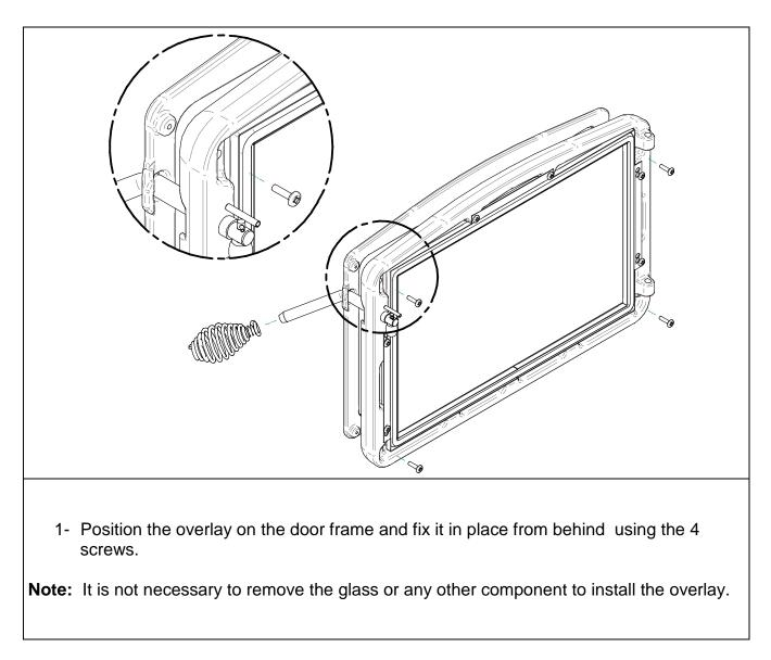
Figure 1.2 Door overlay installation
