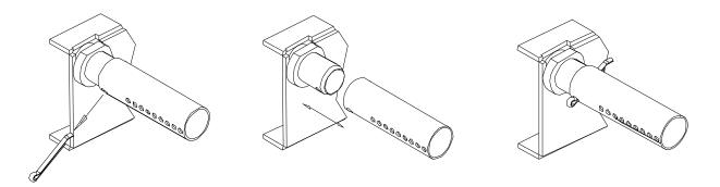
Figure 3.4 – Secondary Air Tube replacement
