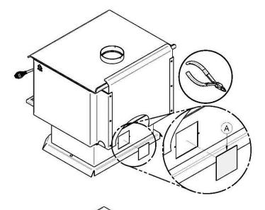
Remove the disposable metal plate (A) behind the pedestal using a pair of pliers.
