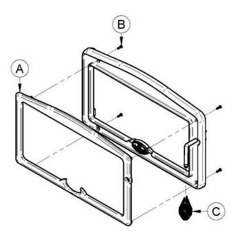
Position the overlay (A) on the door frame and secure it from inside the door using the 4 included screws (B). Install the door handle (C) on the handle rod when finished.
