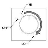
When using the optional blower, allow the stove to reach operating temperature (approximately one hour), before turning it on. The increased airflow from the blower cools the firebox and could affect the start-up combustion efficiency if the blower is turned on too early.
