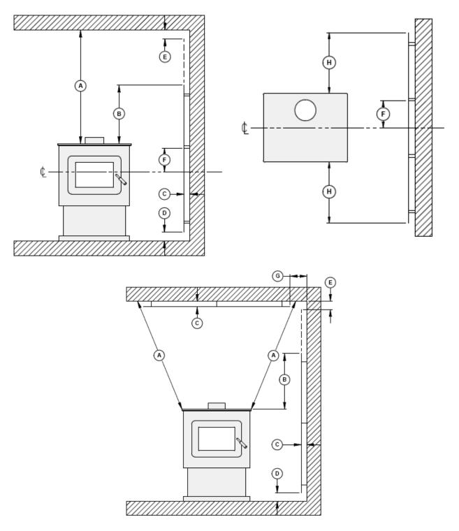
**Clearances for shield construction**
