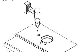
B) You can get from your dealer a liner fixation system (AC02006), sold separately. Follow the installation instructions provided with the liner fixation system.
