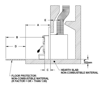
The use of an R value is convenient when more than one material is going to be used in the hearth extension to cover the combustible surface. This is because R values are additive, whereas K values are not.
