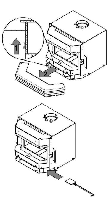
**Step 3:** Remove the lower louvers assembly by lifting it up.
