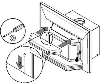
**Step 8:** Put back in place the upper louvers assembly and secure it with the previously removed screw.
