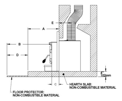
If non-combustible material floor protection needs to be added <u>in front of and level with the hearth extension of the masonry fireplace</u>, an R factor equal to or greater than 1.00 is required.
