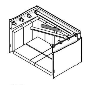
1. Starting with the rear tube, lean and insert the right end of the secondary air tube into the rear right channel hole.
