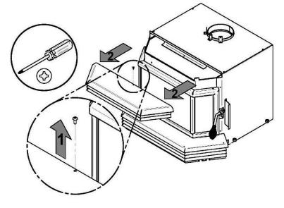
**Step 1:** Using a Philips screwdriver, remove the screw holding the upper louvers assembly.
