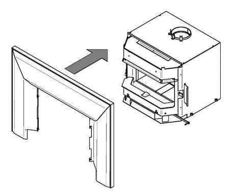
**Step 5:** Install the mounted faceplate on the unit.
