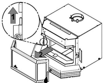
**Step 2:** Remove the door from its hinges.
