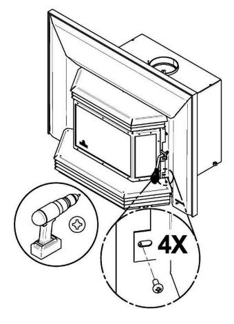
**Step 9:** Secure the faceplate to the unit using four screws #10 x 3/8" provided with the faceplate kit. Make sure the air control mechanism rod moves freely through the lower horizontal slot in the faceplate assembly.
