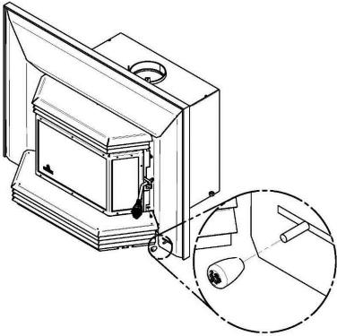
**Step 10:** Install the finish handle onto the air control mechanism rod.
