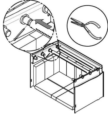
2. Lift and push the tube into the corresponding opposite nozzle. Align both nozzle and tube locking holes together and secure using a cotter pin with a pair of pliers.
